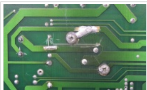
WPC Power/Driver board with C9 connection corrected.
