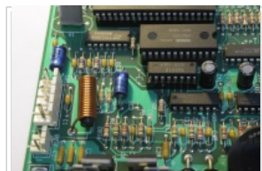
C38 is not stuffed on some pre-DCS sound boards.
