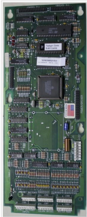
WPC-089 CPU, this one from Twilight Zone, with battery holder removed.
