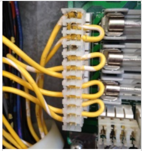
WPC General Illumination Connector J115 (AC power in). Note wire colors, beginning on the bottom with a yellow/white, then three (looped) yellow, then three (looped) yellow/white.
