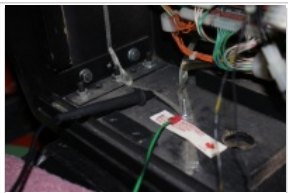
A convenient location to find ground in a WPC backbox.
