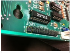
A missing pin in the FlipTonics-to-MPU interface . The missing pin prevented transmission of the F8 signal (D7), which is the upper left flipper switch closed signal.
