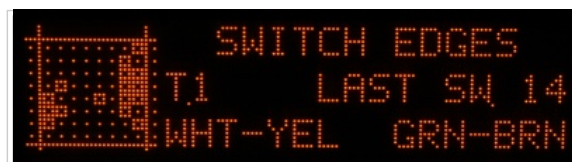
An example switch matrix display, this one from Twilight Zone. Note the opto switches in column 7 (for example) are shown as boxed dots.
