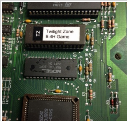
Closeup of WPC-089 MPU that uses a 6264 RAM and a 4M game ROM. Note jumpers W1, and W2 to set ROM size as well as W3 (out) and R93 (in) to set RAM size.
