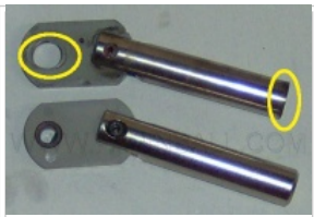
An Example of an Egged Flipper Link and Mushroomed Flipper Plunger - Lower Link and Plunger Shown in Picture is new
