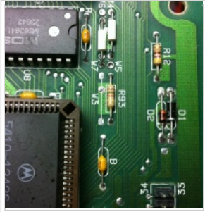
A WPC-089 MPU board with 6264 RAM, jumper W3 removed, and R93 in place.
