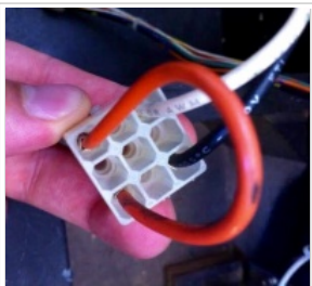
9 Pin WPC Transformer Power Configuration, configured for 230V systems.
