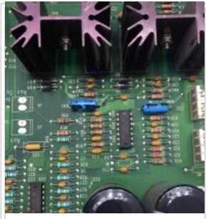
C32 and C41, both electrolytic caps, are in series in the sound amplification circuit of the DCS sound board.
