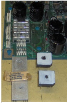
Applying heat transfer grease (heat sink compound) to the new bridge rectifiers.
