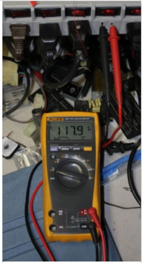
Measure line power at the wall plug that the game is plugged into (not on the bench, as shown here). Almost 118VAC...Nice...
