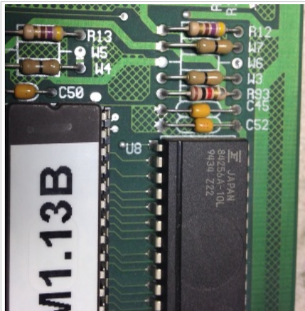
Closeup of WPC-95 MPU that uses a 62256 RAM. Note jumper W3 is installed to set the RAM size for a 62256 RAM.
