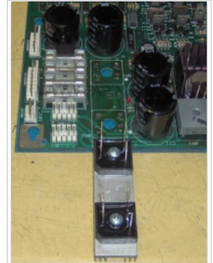
New bridge rectifiers screwed to heat sink before placing on driver board.
