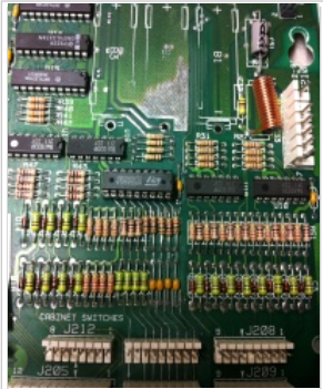
A WPC-089 MPU board, after a couple hours of alkaline corrosion abatement.
