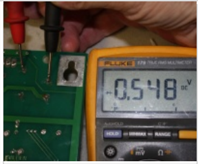
Testing a Bridge Rectifier in circuit. This part of the bridge is good.
