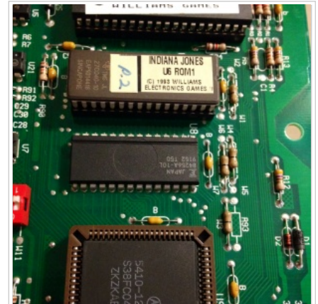
Closeup of WPC-089 MPU that uses a 62256 RAM and a 4M game ROM. Note jumpers W1, and W2 to set ROM size as well as W3 (in) and R93 (out) to set RAM size.
