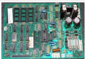
WPC pre-DCS Sound Board, sound ROMs removed
