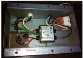
A look inside a typical WPC power box. This particular box was from a Fish Tales. The Thermistor is grey, the varistor is green.
