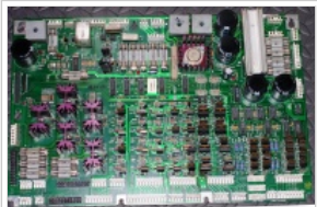
WPC Power-Driver board with Flipper Relay, or the -1 version.
