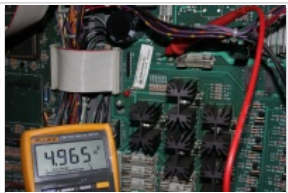
Measuring DC voltage at the 5VDC test point, TP2.
