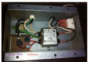
Underside of power box showing varistor and thermistor
