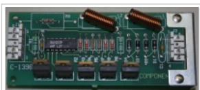
C-13963 High Current Driver board as used in NBAFB and Funhouse.
