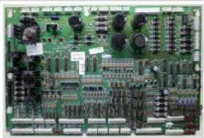
WPC-95 Power/Driver board. This is the later model, with zero ohm jumpers installed in the GI circuit, lower left.
