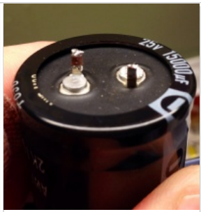
A good view of a 15,000uF cap, with a pulled through hole still on the left lead (the brown donut looking object)
