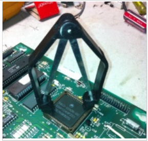
Using a PLCC puller to properly remove the ASIC. Grip firmly, and "rock" the chip out gently.
