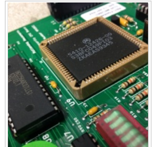
This cracked ASIC socket caused intermittent operation of the game.
