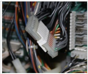
The "Z" connector, as used in Twilight Zone, etc.
