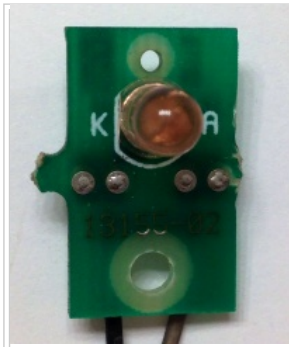
The component side of a typical Williams opto transmitter. When replacing the opto, orient the flat side toward the "K" (equivalently, orient the "short" leg of the opto toward the "K")
