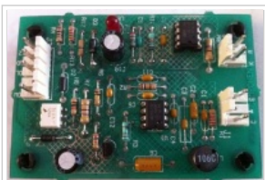
WPC 24 Inch Opto Board as used on BSD and Shadow
