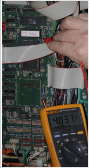
Measuring DC voltage at pin 32 of the game ROM
