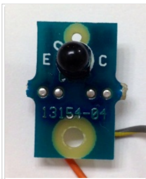
The component side of a typical Williams opto receiver with an aftermarket receiver LED. When replacing the opto, orient the flat side toward the "C" (equivalently, orient the "short" leg of the opto toward the "C"). OEM LEDs have an "ear" that matches the silkscreen on the board
