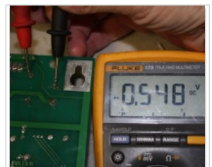
Testing a Bridge Rectifier in circuit
