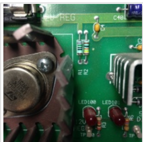
WPC-95 Voltage Adjust resistors R1 and R1
