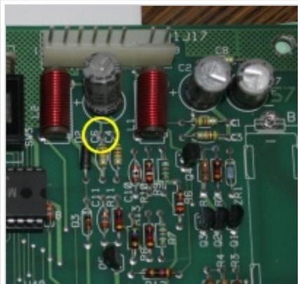
Connect the +5V lead of your logic probe to the top of C6.
