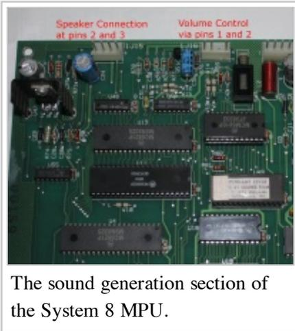
The System 8 MPU creates sound on the MPU itself, much like the baseline version of the System 11 MPU.
