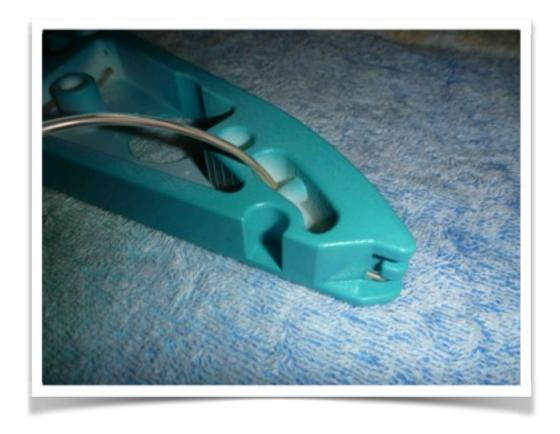
**Step 4** - Before tensioning the el wire feed the remaining EL wire back through the concealed slot and rest in the top groove.
