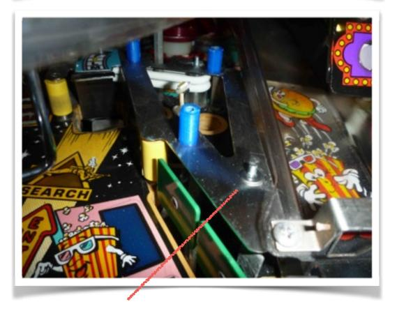
**NOTE**: Using one of the included washers, place it on the post near the two right-side stand up shown with the red line targets before securing the SS plate. You want to make sure that the SS plate is secured well to the post before proceeding.
