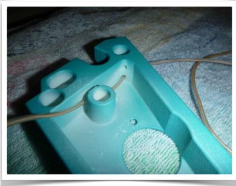
**Step 2** - Lock in the EL wire between the wall and the small vertical cylinder (tension lock) as it has a number of mild indentations to grip the EL wire. Make sure you use a blunt instrument like a plastic ruler to push the el wire into place.
