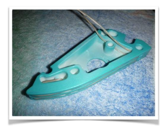
**Step 7** - Using a little force pull the EL wire over the top of the internal tension / lock - check that all slack has been removed from the el wire on the outside for that neat and tight look. Then press the El wire into the locking mechanism using the same blunt instrument to press the El wire into place.
